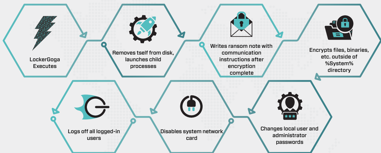
Figure 4: LockerGoga Execution Sequence, Norsk Hydro Variant
